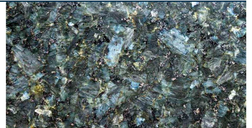
Close up of a polished, dark blue variety of larvikite, also known as “Pub stone”.
